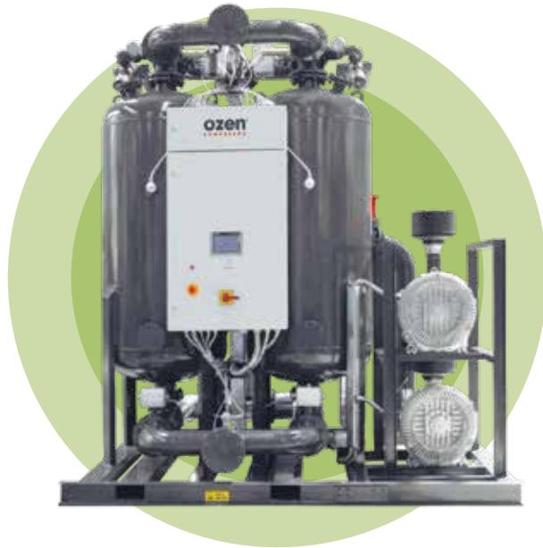
In the OCD-H series heated desiccant dryers, the regeneration of the dehumidifier can be achieved without loss of compressed air by means of centrifugal blower motor and high efficiency heater. The completely automatic drying system uses blower to pull ambient air and pass it through the heater.
